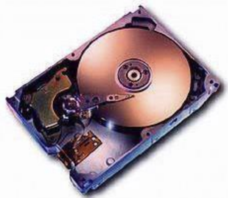
The inside of a typical hard disk
